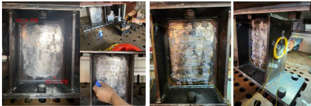
Figure 6: Sensor attachment location(left: DSS, right: DAS)
