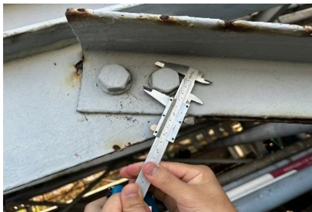
Figure 2: Pipe rack member size measurement
