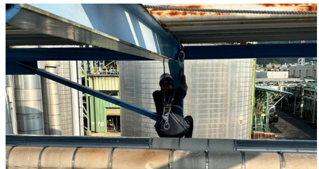
Figure 7: Pipe rack Manpower Excitation Experiment
