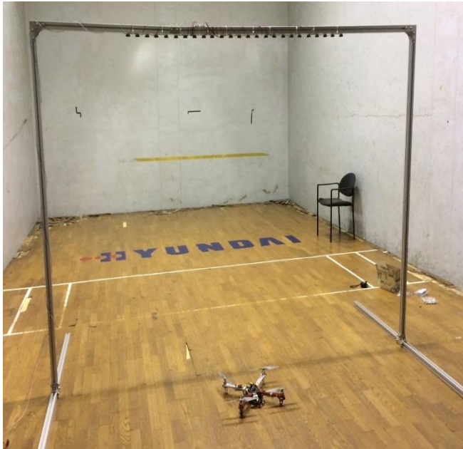
Simple sonic wall (3m-by-2m, 25 speakers)
