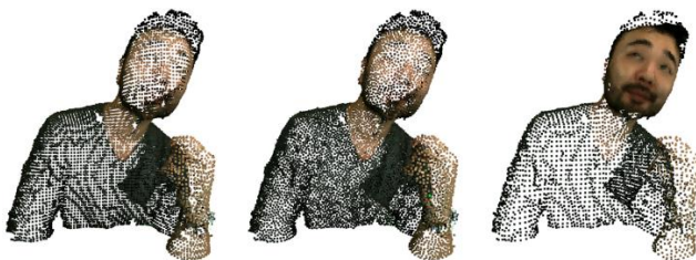
(a) voxel grid downsampling (b) farthest point sampling (c) ROI-preserving downsampling
