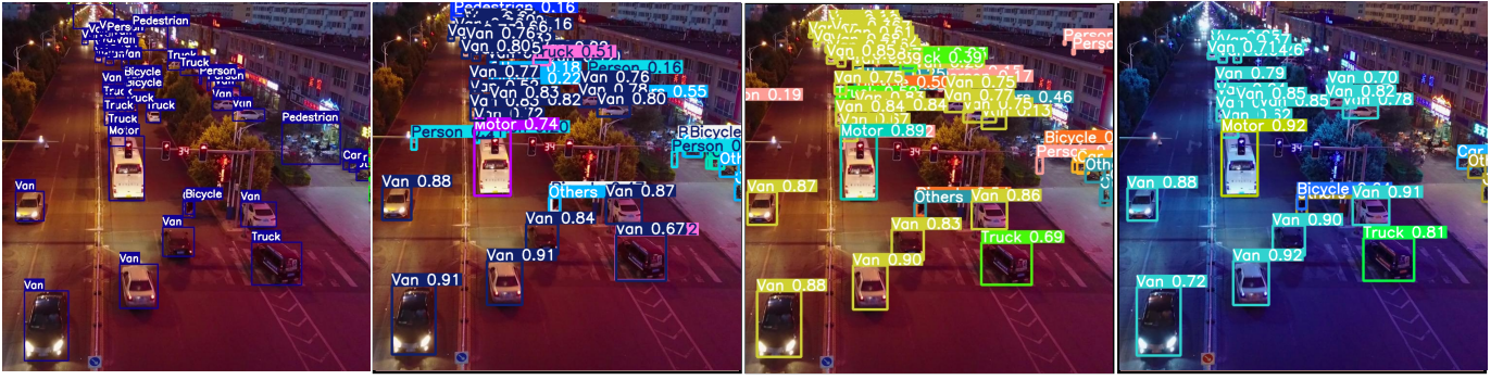
Fig. 2. Comparison of Detection Results Across Models: Ground Truth vs. YOLOv8, YOLOv9, and YOLOv10 on VisDrone Dataset.
