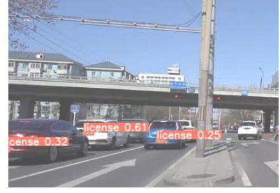
Fig. 2. Real-time test of YOLOv9 trained by multi-vehicle dataset.
