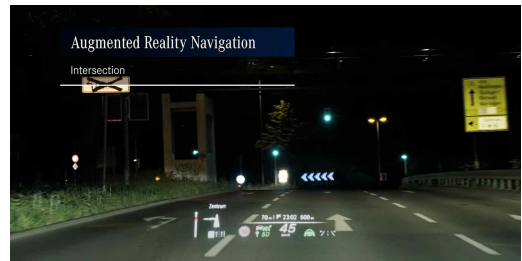
[Fig. 1] AR HUD Mounted on Vehicle
