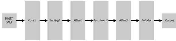
Fig. 2. A proposed CNN Model equipped with BN
