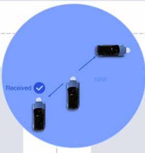
Application-aware, distance-based multicast communication with 5G V2X can assist in intersection management
