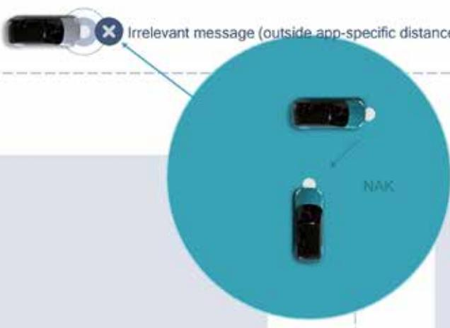
Application-specific distance is determined based on relevancy
