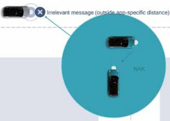
Application-aware, distance-based multicast communication with 5G V2X can assist in intersection management
