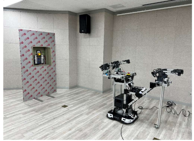
Fig. 3. Teleoperation framework with distribution panel testbed
