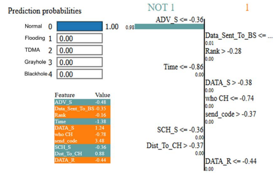
Fig. 8: The model predicts NOT-1 (Normal) on WSN-DS dataset with 100% probability, mainly due to strong opposing evidence from teal-highlighted features (ADV_S, Time, SCH_S, Dist_To_CH).
