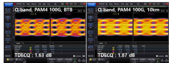
Fig. 2. EYE diagrams of normal IA-EML with PAM4 100 Gbps modulation for BTB and 10 km transmission at 50 °C.
