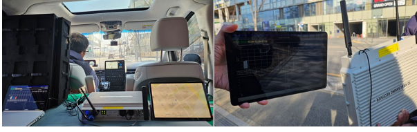
Fig. 2. On-Site Measurement and Custom-Developed 5G Scanner
