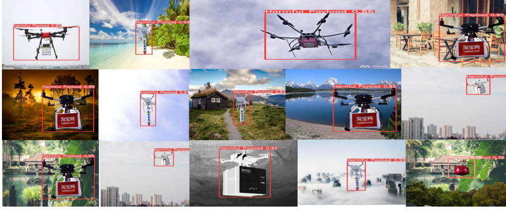
Fig. 3: Inference result using test dataset showing object detection of UAV carrying harmful payload
