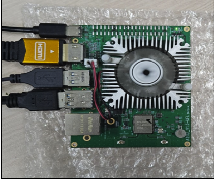
Fig. 4: Custom Build Lightweight Edge Device for Edge Deployment and HMC Monitoring.
