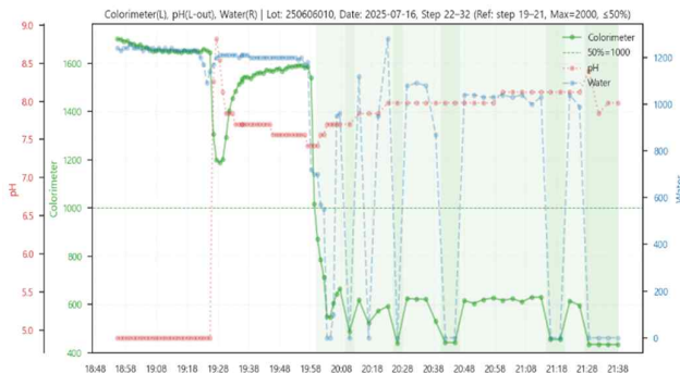
Figure 4. Composite sensor that consists of colorimetry and pH sensors: rinsing-process results for dark-shade dyeing.
