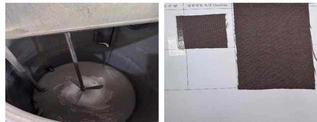
Figure 1. Assessment of rinsing completion of dyed fabrics by visual inspection
