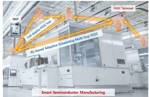
Fig. 1. Concept of RL-based adaptive scheduling in a full-duplex multi-hop FSOC network under OHT blocking events in smart semiconductor manufacturing.
