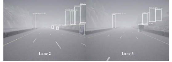
Fig. 8: Example of an adaptive lane change maneuver performed due to close-proximity risk detection, leveraging V2V lane occupancy information.
