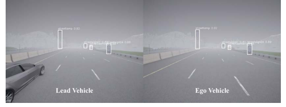
Fig. 7: Ego vehicle and lead vehicle camera view in fog with object detection.
