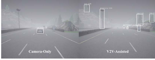
Fig. 9: Comparison of perception range and safe following distance between a Camera-Only YOLO system and the proposed V2V-Assisted system in foggy conditions.
