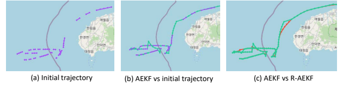
Fig. 2: Comparison of reconstructed vessel trajectories. (a) Initial AIS data with missing segments; (b) AEKF-based reconstruction vs. raw data; (c) Enhanced reconstruction by R-AEKF.
