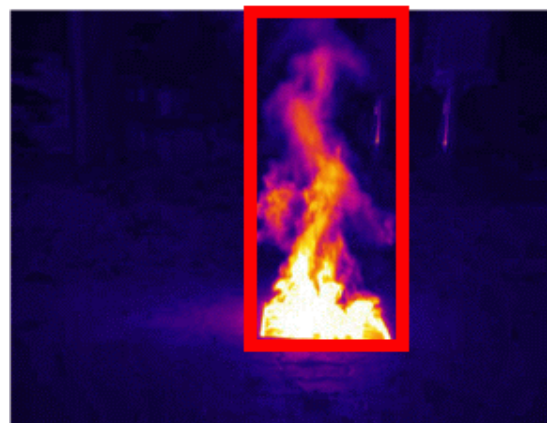
Fig. 2. An example of thermal image data labeling
