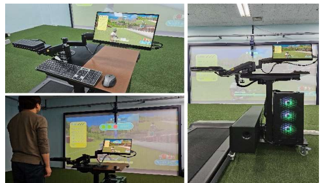
Fig. 2. A large screen-based headset-free XR system for barrier-free XR contents.
