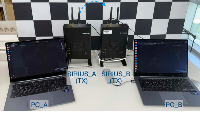
Fig. 4. SIRIUS 5G-V2X testbed.
