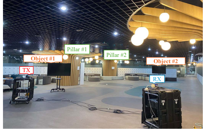
Fig. 1. The experiment layout for 28 GHz indoor measurements.
