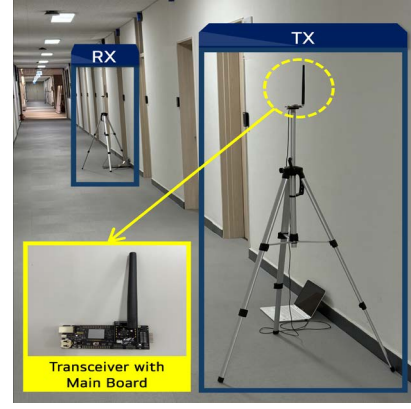
Fig. 2. TX and RX setting for channel measurements.
