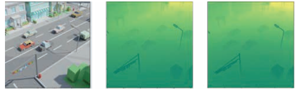
Figure 6: Synthetic generation of outdoor scene data, including RGB images, depth information, and object distance mapping.
