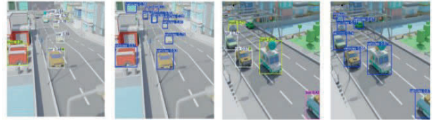
Figure 5: Visulaization of object detection results on synthetic data, demonstrating accurate detection and identification of vehicles at varying distances.
