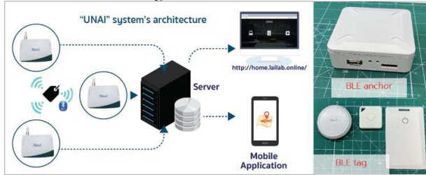
Fig. 1 BLE architecture system with an Anchor and tags.
