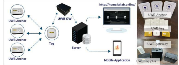
Fig. 2 UWB system architecture with a picture of the Anchor and tags
