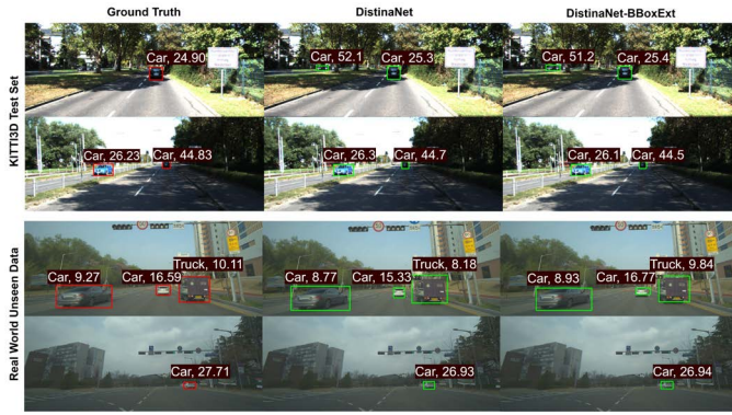
Fig. 6. Qualitative results of the presented DistinaNet and DistinaNet-BBoxExt models in both KITTI test set and collected unseen real-world images. The values are presented in meters.
