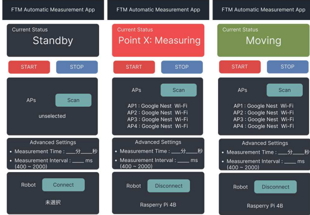
Fig. 7. User interface of the FTM automatic measurement application.
