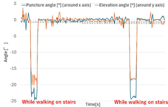
Fig .9. Change in odometry during level and stair walking.
