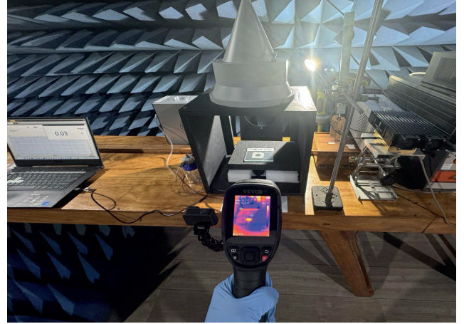
Fig. 1. Testbed during test which is connected with a laptop to collect the result from the RadMan2 receiver.
