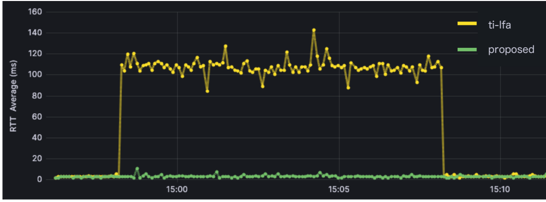
Fig. 4: Visualization results: TCA caused a latency at 14:58 and resolved at 15:08. During that time, a lower-latency backup path existed compared to the path provided by TI-LFA.
