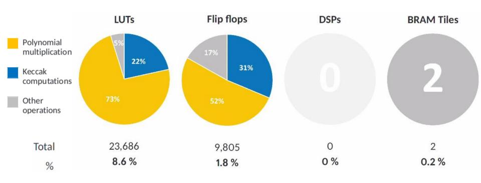
In one FPGA: 11 coprocessors can be fit  $\rightarrow$  504 K / 416 K / 342 K KEMs per sec
