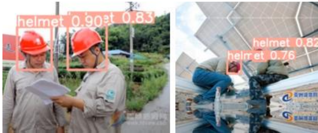
Fig. 6. Deep learning model test results based on YOLOv5 in google colab environment
