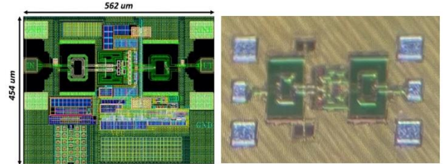
Fig. 6 Layout and microphotograph of proposed phase shifter
