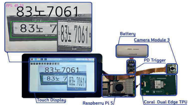
Figure 4. Operation Screen of the Proposed Real-Time Portable License Plate Recognition System
