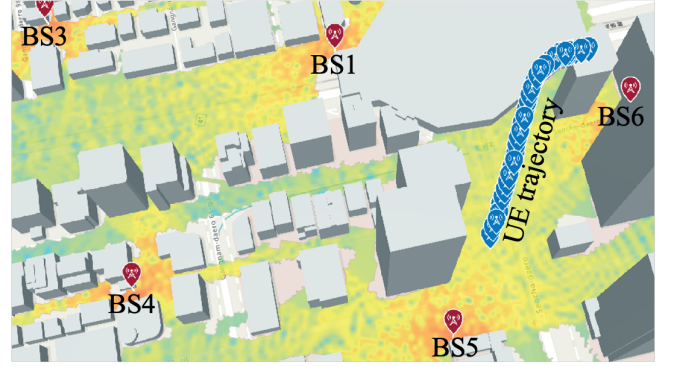
Fig. 1. mmWave outdoor Urban Micro Street Canyon deployment scenario with a UE mobility trajectory
