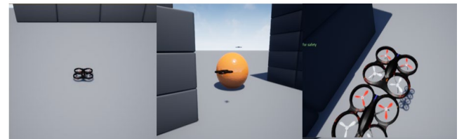
Figure 1. Airsim Simulation. (a) Initial State; (b) Tracking; (c) Interception.
