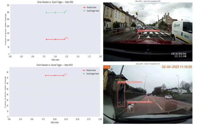
Fig. 2: Visualization of multi-modal real-time hazard detection with VLM-based captioning.
