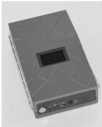
Fig. 1 Photo of the portable black carbon measuring instrument
