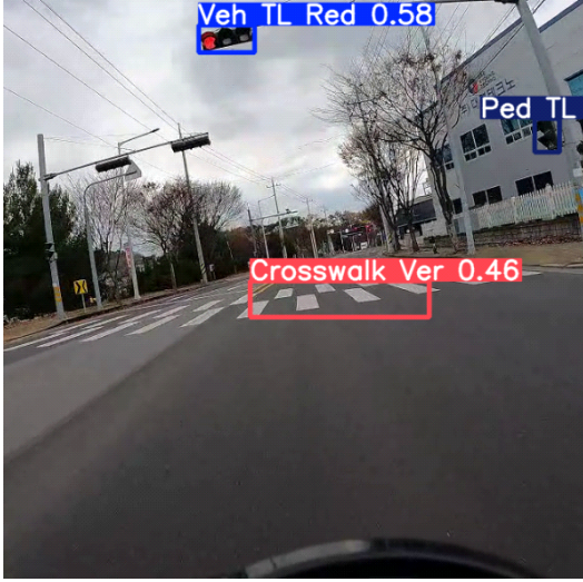
Fig. 5. Example of a red light being detected while the stop line is missed after vehicle passage
