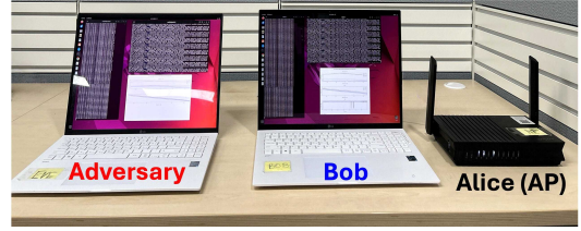
Fig. 4. Experiment setup: NETGEAR AX1800 (RAX20) model used as AP (Alice) and two laptops equipped with Intel AX201 NIC used for Bob and the adversary
