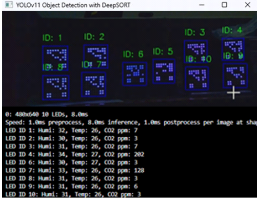
Fig. 7. Multi-tracking mechanism based on the DeepSORT algorithm.
