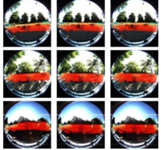
Fig. 3. Estimated extrinsic calibration using the proposed deep learning model. From left to right, each row shows the initial misalignment, ground truth, and calibrated image results.
