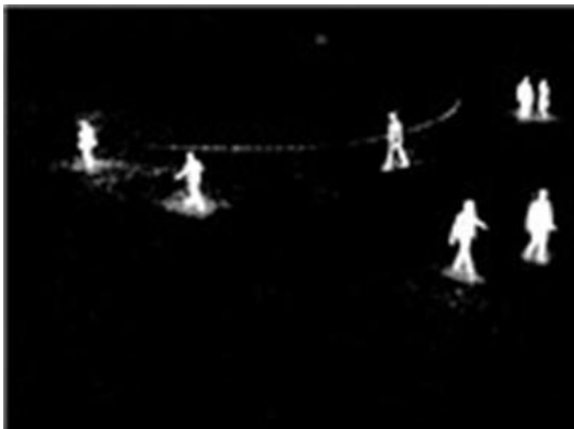
Fig. 2. An Example of Background Removal Using BackgroundSubtractorGMG.
