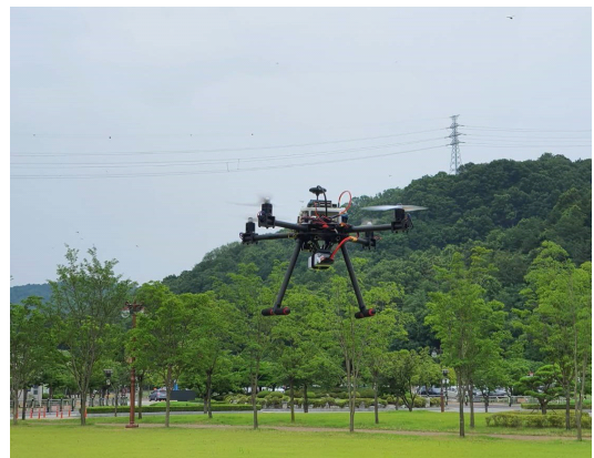
Fig. 8. Outdoor flight test of the UAV equipped with the Active Noise Cancellation (ANC) system.
