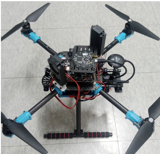
Fig. 7. UAV hardware setup for testing the Active Noise Cancellation (ANC) system: The platform includes an Nvidia Jetson NX for real-time processing, ReSpeaker Mic Array for noise capture, and speakers for anti-noise emission, enabling effective reduction of propeller noise.
