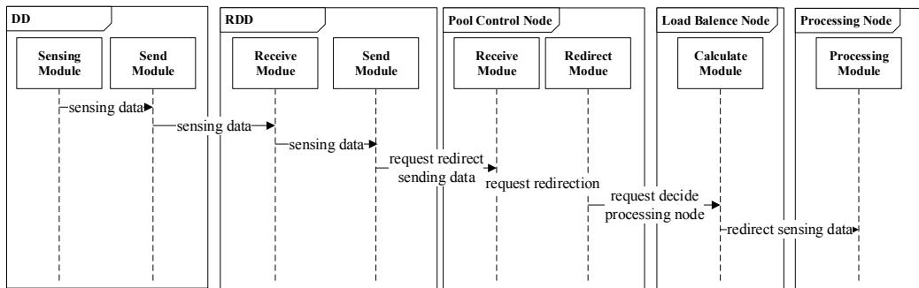
**Fig. 2.** Flow of data processing in the entire system.
