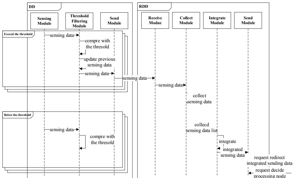
**Fig. 3.** Flowchart of the filtering processing work.
