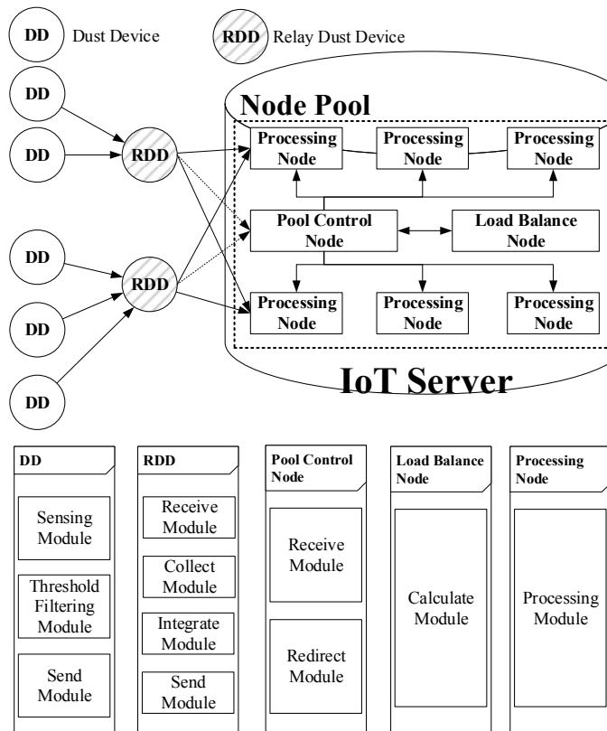
**Fig. 1.** Overview of the 3-layered hierarchical smart dust system.
