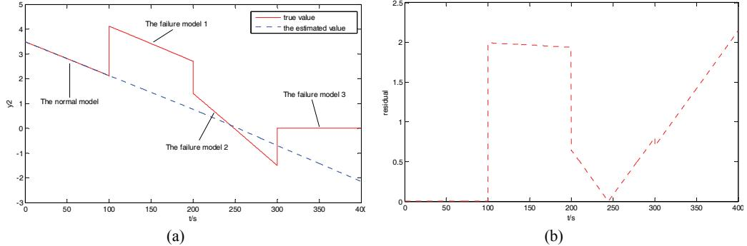
**Fig. 2.** (a) The tracking results and (b) the residuals for fault status  $y_2$  using CRPF in Experiment 2.
