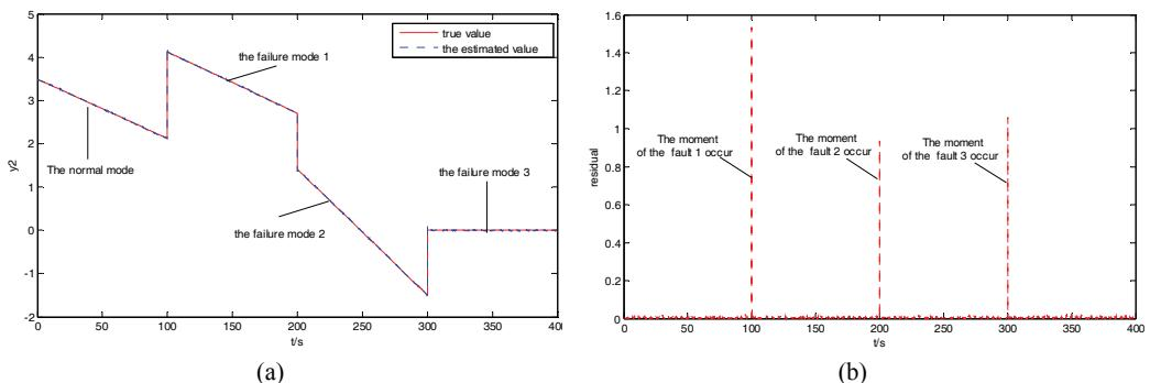
**Fig. 3.** (a) The tracking results and (b) the residuals for fault status  $y_2$  using the proposed method in Experiment 1.
