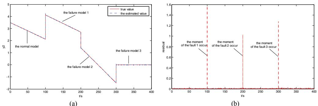
**Fig. 4.** (a) The tracking results and (b) the residuals for fault status  $y_2$  using the proposed method in Experiment 2.
