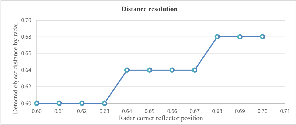
Fig. 12. Demonstration of distance resolution tested from the detected object distance by radar.
