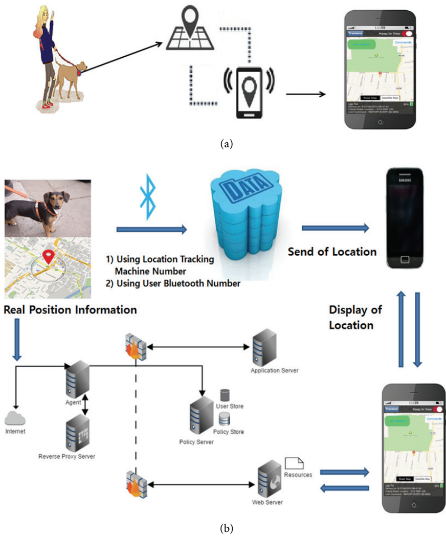
Fig. 5. Real-time animal localization system for animal care using GPS and Bluetooth. (a) Bird's-eye view diagram. (b) Service diagram.
